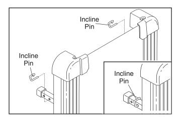
CAUTION: Before using the treadmill, make sure that both incline legs are at the same height. Do not use the treadmill with the incline pins removed. After you have adjusted the incline legs, lower the treadmill (see HOW TO LOWER THE TREADMILL FOR USE on page 15).
